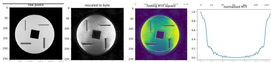
Figure 1. Output images of Hazen spatial resolution analysis using MTF method.
